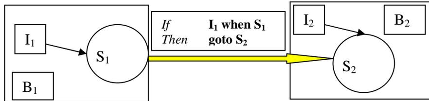
Figure 10. Concept for State Transition using Process Rules
