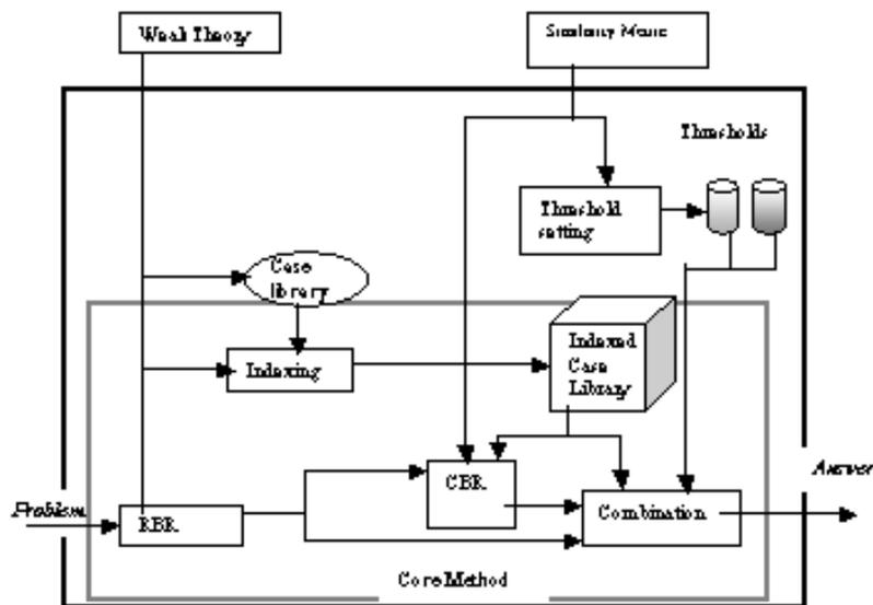
Figure 9. NCODES Integrated Rule / Case System Architecture
