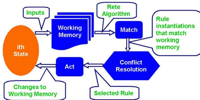
Figure 11. Concept for State Transition Flow
