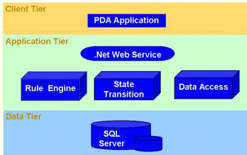
Figure 8. NCODES Conceptual Multi-Layered Architecture
